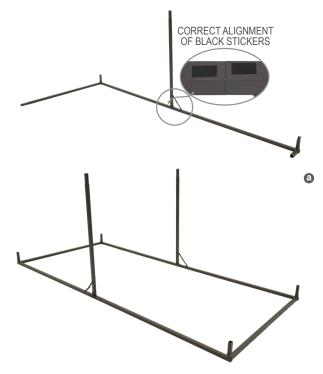
2. After each section is identified, connect the two base frame a sections together by connecting all black stickers together.
